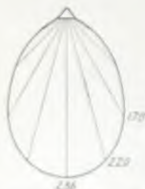
Distribution of light from the No. 700 Reflector, with a 60-watt Mazda Lamp
